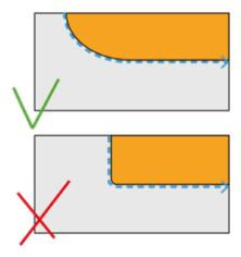
If the piece has curves with a radius under 10 mm:
