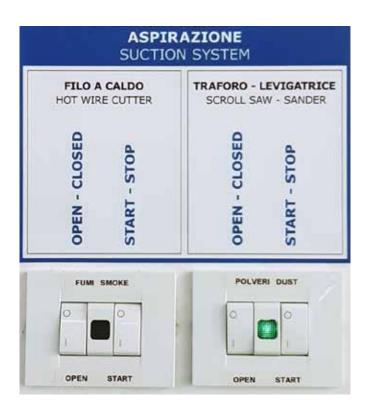
**Open the lower shutter**, located on the suction pipe in correspondence to the machine you want to use, turning it to a vertical position.
