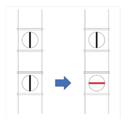
Reset the OPEN and START switches on the dust aspiration system.
