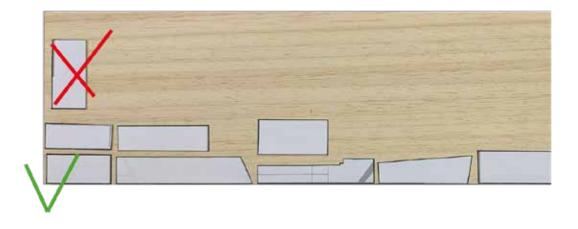
If you need to cut several pieces, we recommend cutting out the shapes from a printed drawing and applying them directly to the board with removable double-sided adhesive tape at a distance of 2 or 3 mm from each other to allow the blade to pass through and optimize the number of cuts to make.
