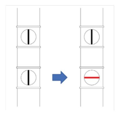
Reset the two OPEN and START switches on the dust extraction system.
